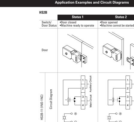
0 🖂 Θ O Main 3-4: Closed 3-4: Open Circuit Aux. 1-2: Open 1-2: Closed Circuit 1. Main Circuit: used to enable the machine to start only when the main
